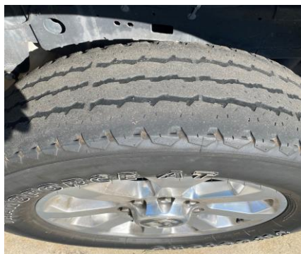
A dangerously illegal tire still in use
